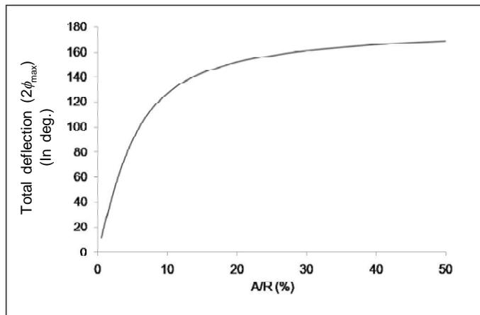
**Figure 3.** The ratio of sinusoidal path amplitude  $A$  and radius  $R$  of circular path determines the total angle of deflection  $2\phi_{\max}$ . The depicted plot is for  $\theta_0 = 18^\circ$ .
