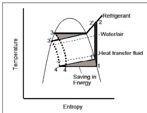
**Figure 4.** The shaded area gives the energy savings due to glide-matching when zeotropic refrigerant mixtures are used in a Lorenz–Meutzner cycle (1'-2'-3'-4') and glide of the refrigerant is close to that of the heat transfer fluid, compared to a refrigerator operating with a pure fluid as the refrigerant and the Clausius–Rankine cycle (1-2-3-4).
