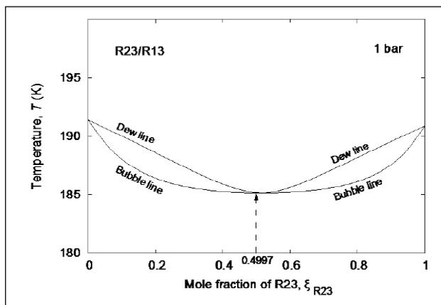
azeotropic mixtures used in refrigeration industry is lower than the constituents of the mixture. Since azeotropic mixtures allow reaching temperatures lower than those with pure single component fluids, these have long been used in the refrigeration industry.
