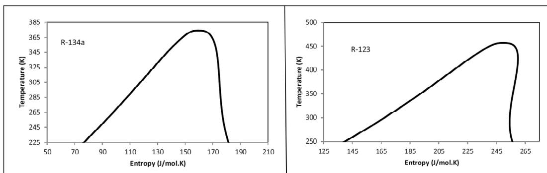
**Figure 5(left).** Vapour dome of a typical refrigerant (HFC134a) with negative slope of the saturated vapour line.
