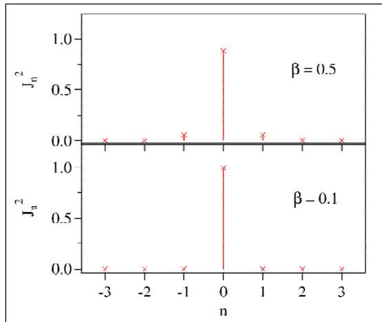
**Figure 1.** Spectral intensity of center and sidebands in fm modulation for two values of the modulation index  $\beta$ . The sidebands are practically zero for  $\beta = 0.1$ .
