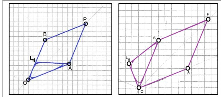
OB. Irrespective of the angles made by OA and OB with the horizontal,  $OL_3$  is always positioned such that  $\angle L_3Ox = \angle AOx$  (which is  $\theta$ ) +  $\angle BOx$ , (which is  $\psi$ ).
