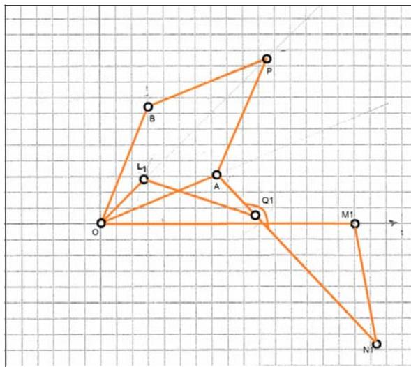
3. Locate hinge  $M1$  on the  $x$ -(horizontal) axis at a distance of 4 units. Hinge  $M1$  is also fixed.
