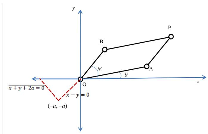
Let us choose a simple curve  $\mathcal{C}(x, y)$ . The point P on the parallelogram is expected to trace the dotted curve shown in *Figure 8*. The curve is composed of two lines whose equations are  $x - y = 0$  and  $x + y + 2a = 0$  for some  $a$ , and the lines intersect at point  $(-a, -a)$ . Multiplication of these two equations yields
