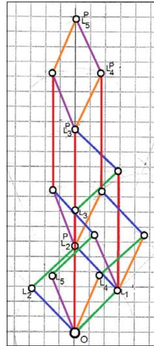
**Figure 13.** Links  $OL_i$  translated to get the extreme point  $L_5^P$ . The parent parallelogram  $OAPB$  is not shown.
