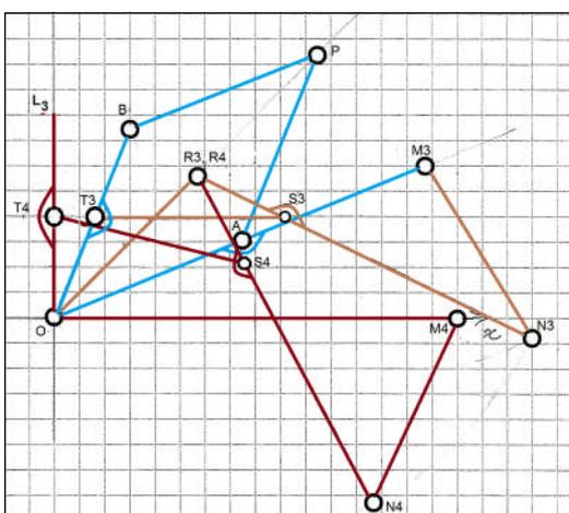
**Figure 11.** Orienting link  $OL_3$  via Kempe's additor.  $OL_3$  sums the angles made by links  $OA$  ( $OM3$ ) and  $OB$  with link  $OM4$ .
