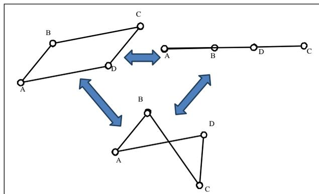
**Figure 6. Possibility of a parallelogram degenerating into a straight line or a contra-parallelogram while the linkage is in motion.**
