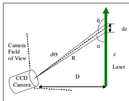
An air parcel at height  $z$ , with altitude range  $dz$ , located at a range (slant distance)  $R$  from the camera is imaged by a pixel<sup>6</sup> with field of view  $d\theta$ . The scattering angle, which is the angle between the
