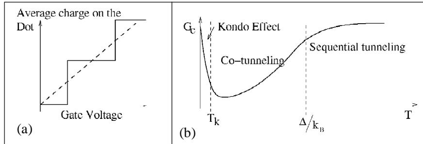
**Figure 2. (a) Coulomb Staircase showing the single electron transfer; at high temperatures  $k_B T \gg e^2/2C$ , this Coulomb blocking vanishes and the average charge on the dot varies linearly with the applied gate voltage (dotted line). (b) Conductance vs temperature for the quantum dot;  $\Delta = e^2/2C$  is the electron charging energy (adding or removing of one electron), and  $C$  is the dot capacitance.**
