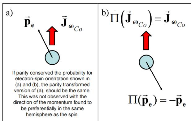
**Figure 2. Schematic (a) is of the direction of the  $\beta$  decay electron, characterized by momentum  $\vec{p}_e$ , with respect to the spin of the  $^{60}\text{Co}$  nucleus,  $\vec{J}_{^{60}\text{Co}}$ . Schematic (b) is the same process transformed by the parity operation. Unequal probabilities for these two processes to occur were observed by Wu and collaborators; this was the first experimental evidence for parity violation in nature.**
