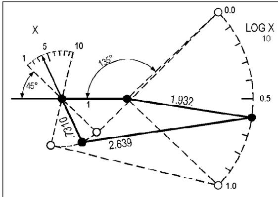
**Fig. 2. Three-Point Approximation for Log Function.**
