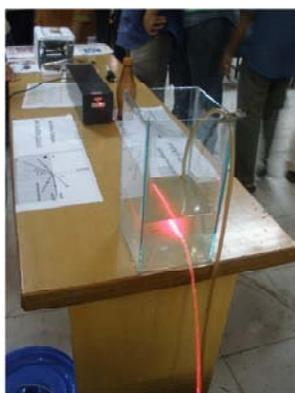
8 mm in one side at a height of 70 mm from the bottom. Fill the tank with water to a height of about 200 mm. There should be a steady stream of water, which can be collected in a bucket and resupplied to the container. Now if you direct a laser beam (from a low-cost laser pointer) at the stream, you will find that it gets guided along the parabolic path of the water due to total internal reflection. Voila! You have just made an optical water waveguide.
