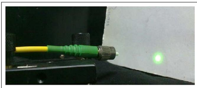
**Figure 3. Single-mode fiber cable used for transporting green laser light. The cable is terminated with a fiber connector (green strain relief and silver nut) that allows us to connect the beam to the experimental apparatus. The actual fiber is covered with a yellow furcation tubing seen on the left. Note the perfect modal quality of the output beam falling on the white card.**
