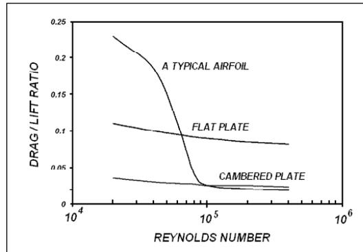
**Figure 4. Critical Reynolds number of airfoils: The drag to lift ratio of a typical airfoil drops rapidly around a Reynolds number defined as its critical Reynolds number. This number depends on the profile of the airfoil but is typically around 50,000. Flat and curved plates with a small thickness ratio of 2% do not show this behavior.**
