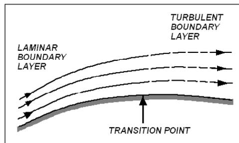
the airfoil, the nature of flow is similar to the above, but the transition point moves somewhat upstream. There may also be some flow separation on the top surface as we approach the trailing edge. The drag of the airfoil in this condition is mainly due to skin friction in the boundary layers and is small. The ratio of lift to drag is high.
