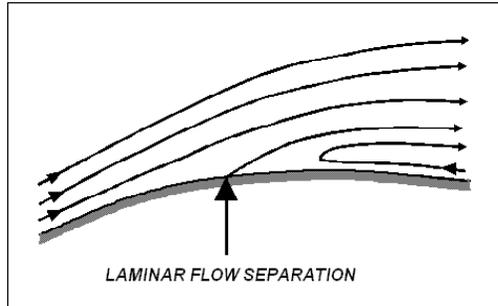
to the air-foil surface. This leads to a large region of separated flow as illustrated in *Figure 3*. The airfoil drag is high due to low pressure in the separated region.
