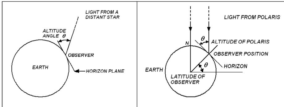
**Figure 2 (left).** The altitude of a star: The altitude of a star is the angle made by the line of sight of the star with the horizontal plane at an observer’s location on Earth. This angle can be measured by an optical instrument called the sextant.
