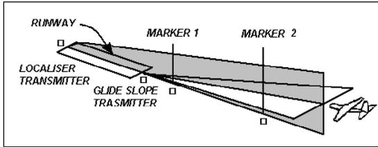
**Figure 8. Operating principle of the ILS:** The ILS system transmits a pair of signals for the indication of flight path deviation from the designed glide slope of 3° and another pair for the indication of the flight path deviation from the centre line of the runway. The pilot notes the deviations on the ILS instrument on board and
