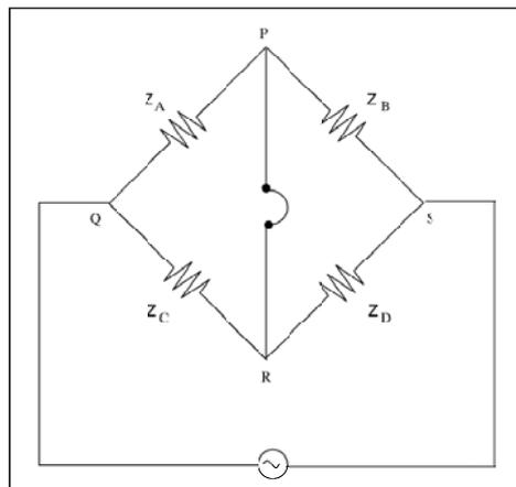
**Figure 2. A simple Wheatstone Bridge arrangement.**
