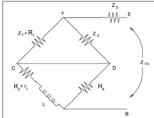
itive in nature, i.e., of the form of  $a - jb$ . The Thevenin impedance of the Anderson Bridge circuit ( $Z_{TH}$ ) as seen by the headphone is theoretically determined by shorting the AC source (i.e., neglecting the impedance of the source), giving (see *Figure 4*)
