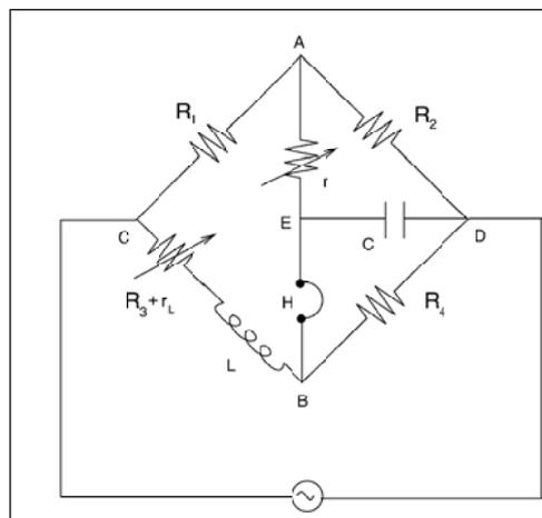
**Figure 1.** The circuit schematics for Anderson Bridge. The resistance  $r_L$  is the resistance of the coil whose self-inductance is being determined.
