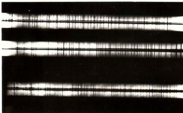
In 1911, Evershed put into operation a second spectroheliograph as an auxiliary to the Cambridge instrument utilising its perfect movement and using a grating and special arrangements for getting photographs of the solar disk in H-alpha. As red-sensitive plates became available, he started obtaining daily spectroheliograms in H-alpha along with the same in the Ca II K line.
