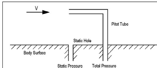
**Figure A. Measurement of static and total pressures. The fluid flow past a small hole in a wall slips past leaving the fluid in the hole at rest. The pressure in the moving fluid is transferred to the fluid in the hole and this is conducted to the measuring instrument. But in the case of the pitot tube, the fluid decelerates ahead of the opening and comes to rest at the opening. The pressure indicated is the total pressure.**
