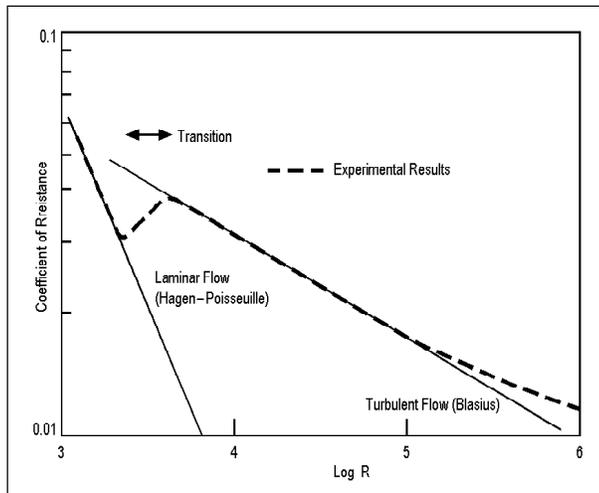
**Figure 4. Frictional resistance of smooth pipes. At a Reynolds number below 2000, the flow is laminar. At a Reynolds number over 4000, the flow is turbulent and the resistance is much larger than in laminar flow. There is a small range over which the transition occurs.**
