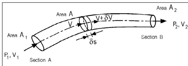
**Figure 2. Flow of an ideal fluid along a stream tube. The fluid element is accelerated by the force due to the pressure difference between its ends. Viscous forces are absent.**
