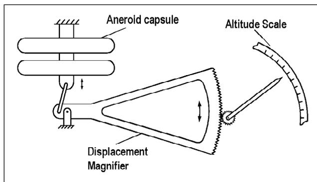
**Figure A: The pressure altimeter.**
