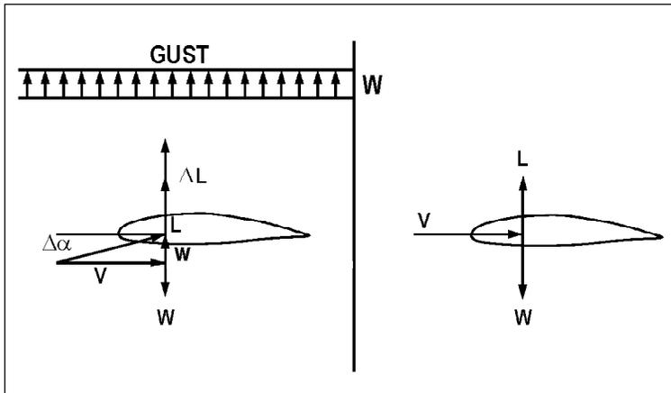
**Figure 3. A wing penetrating a gust: There is a sudden change in incidence and a corresponding change in lifting force. This induces a transient motion of the airplane during which there is a vertical acceleration and this causes discomfort to passengers and also imposes additional loads on the wing.**
