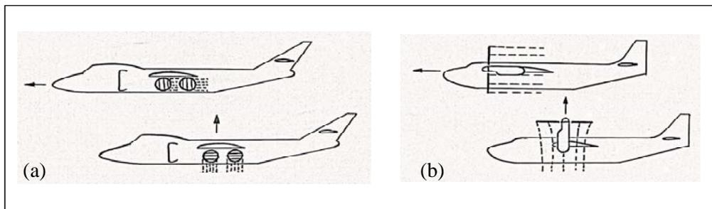
**(a) Tilt rotor:** Vertical take off and landing is achieved in this airplane by tilting the engines such that the propeller thrust is vertical. During normal operation, the propeller provides forward thrust as in a conventional airplane.
