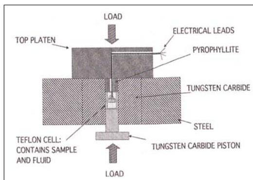
**Figure 1. Schematic diagram of a piston-cylinder apparatus with teflon cell for measuring electrical resistivity of materials under high pressure and temperature.**
