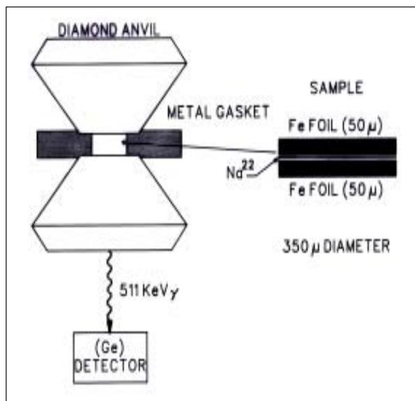
**Figure 8.** Experimental configuration for positron annihilation studies under high pressure using a DAC.
