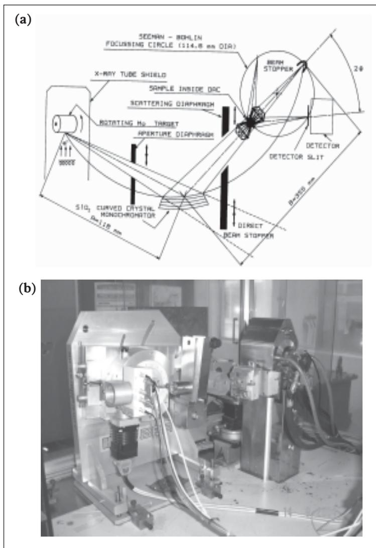
**Figure 4. (a) Schematic and (b) photograph of the high pressure powder ADXD system using a DAC in Guinier geometry.**
