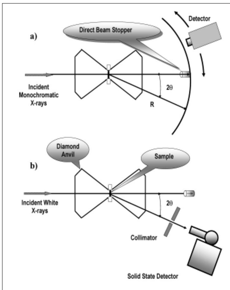
*Figure 3. X-ray diffraction in (a) angle dispersive (ADX) and (b) energy dispersive (EDXD) geometry.*
