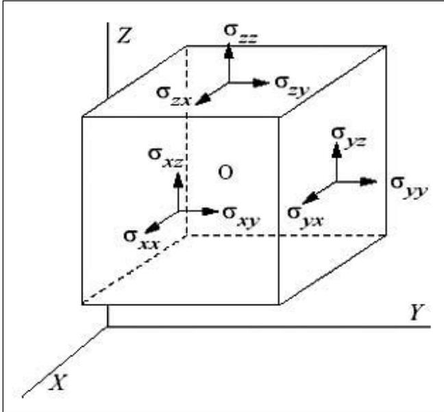
Figure 1. Infinitesimal material cube showing the nine components of the stress tensor.
