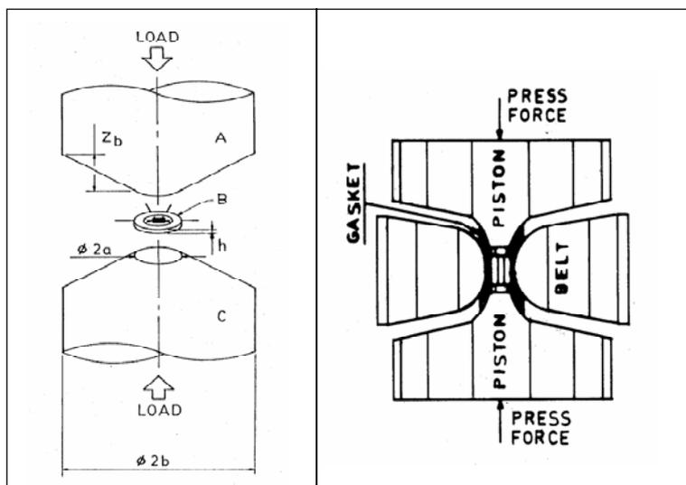
**Figure 5 (left).** Schematic layout of the opposed anvil device. A: upper anvil, B: gasket, C: lower anvil.
