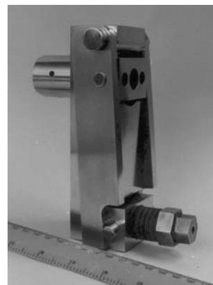
**Figure 9.** Photograph of the Mao-Bell type DAC designed and fabricated at IGCAR.
