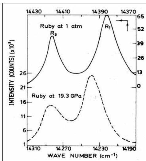
**Figure 14.** The Ruby fluorescence spectra at 1 atmosphere and 19.3 GPa.
