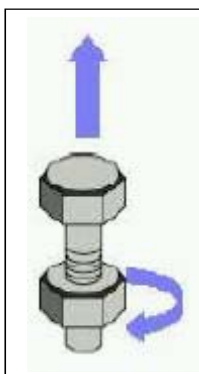
Figure 9. The rotation of the nut in the direction shown causes movement of the bolt in the direction indicated by the straight arrow.
