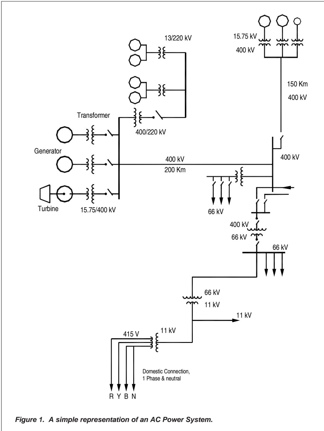
Figure 1. A simple representation of an AC Power System.
