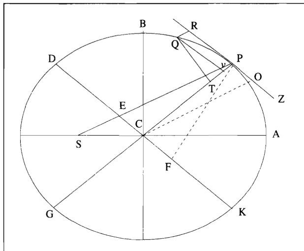
**Figure 3.** Diagram to compute centripetal force directed to the centre or the focus of an elliptical orbit.
