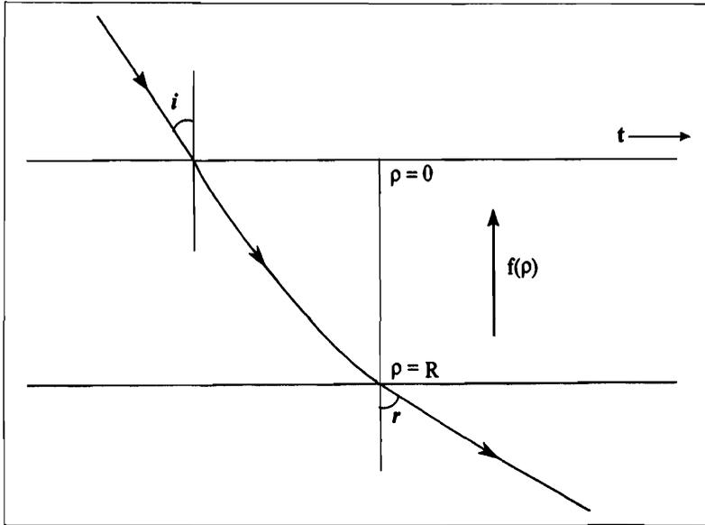
**Figure 4.** Newton's derivation of Snell's Law of Refraction (the ray shown is from denser to rarer medium).
