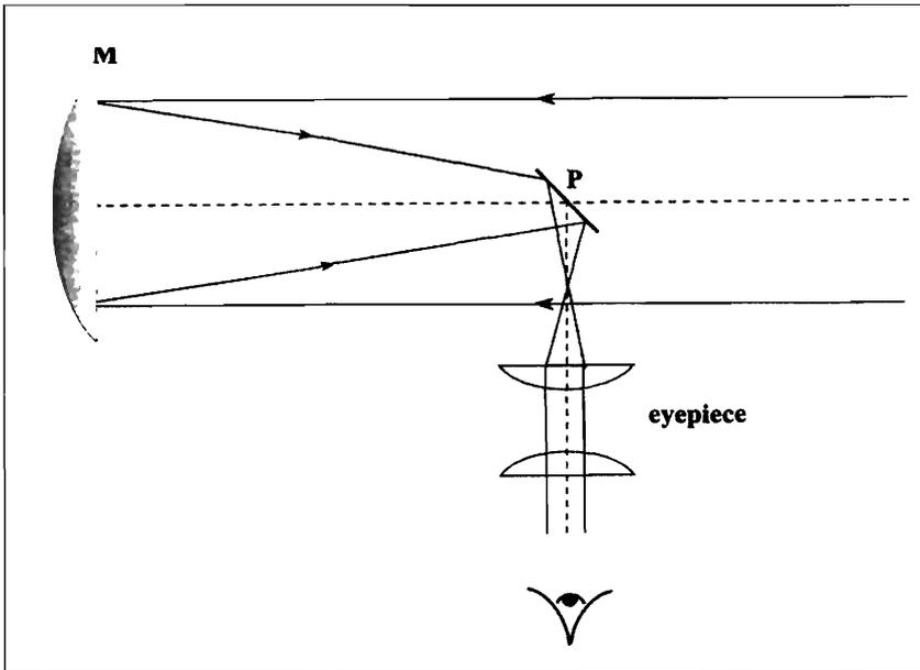
*Figure 2. Schematic diagram of Newton's reflecting telescope.*
