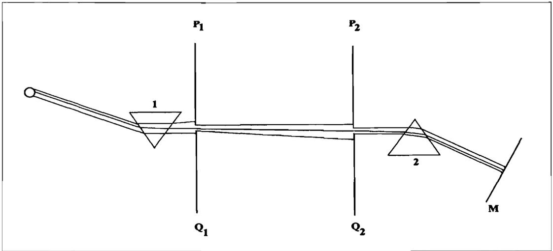
**Figure 1.** Newton's 'experimentum crucis' showing that colours are not created by refraction, but exist in white light. The two slits  $P_1, Q_1$ , and  $P_2, Q_2$  are about 4 m apart. Light beam entering through the shutter falls on prism 1. As the prism is rotated axially, pure colours appear in succession at different points on the screen at M.
