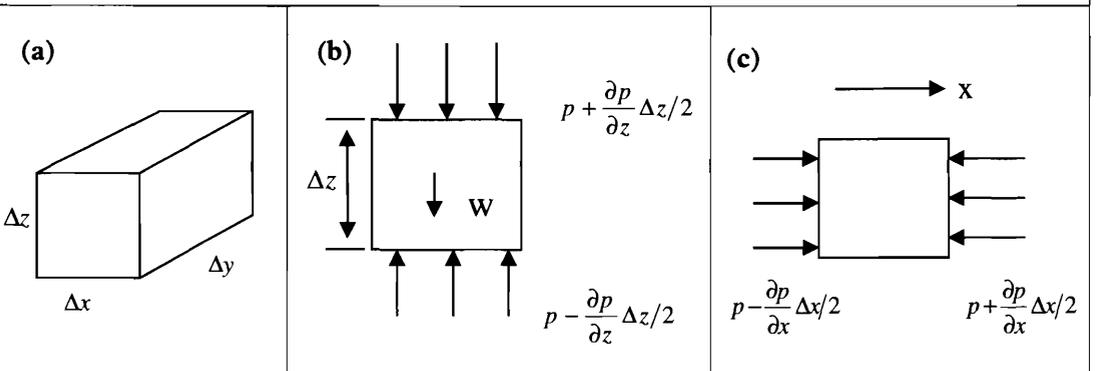
**Equilibrium of an elemental volume (a) in the vertical direction (b) and in the horizontal direction (c). Pressure increases with depth to support the weight and does not vary in the horizontal direction.**
