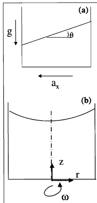
**Figure 3.** (a) Top. Free surface tilts when the container accelerates in the horizontal direction  $\tan \theta = a_x / g$ . (b) Bottom. A liquid in a rotating container rotates as a rigid body. The free surface is a paraboloid of revolution.
