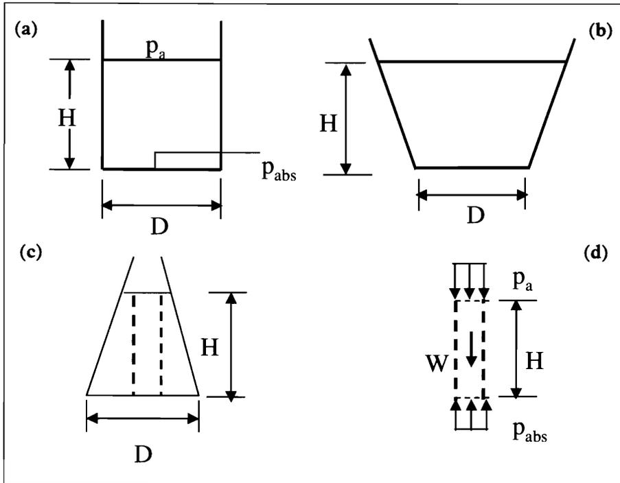
**Figure 1. Pressure on the bottom surface is same in all the three containers. Equilibrium of vertical slice (d) shows that  $p_{abs} = p_a + \rho g H$ ; note that shear stress is zero.**
