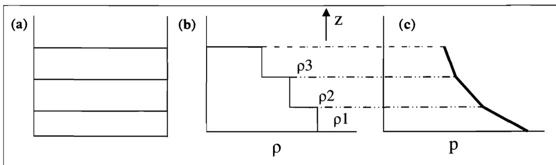
**Figure 2.** (a) Three layers of immiscible liquids. (b) The variation of density with height. For equilibrium, the interfaces between the liquids have to be horizontal. From stability considerations the heaviest liquid is at the bottom and the lightest at the top. (c) The pressure increases linearly in proportion to the density in each layer.
