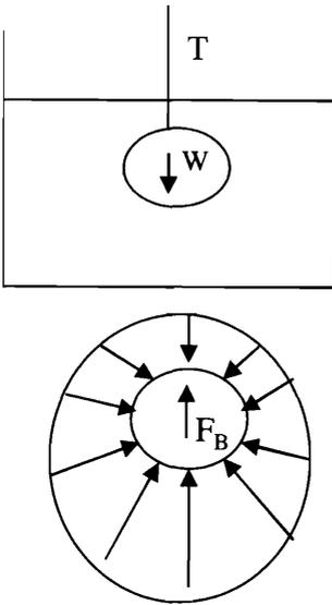
**Figure 4.** A body immersed in a fluid feels an upward force  $F_B$  due to the pressure increasing with depth. There is no horizontal force, pressure acts normal to the surface at each point. The tension in a string supporting a body is  $T = W - F_B$ .
