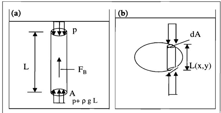
**Figure 5.** a) Derivation of Archimedes principle for a submerged vertical cylinder  $F_B = \rho gLA = \rho gV$ . b) For an arbitrary body integration over 'elemental' cylinders gives the Archimedes buoyancy force.
