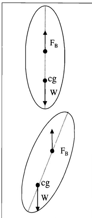
**Figure 7.** For stability of a fully submerged body the centre of gravity (cg) should be below the centre of buoyancy. Any tilting will give a righting movement.
