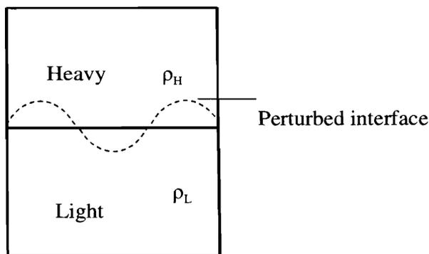
**Figure 6.** A heavier fluid over a lighter fluid can be in equilibrium, but it is not stable. A small perturbation of the interface (shown in dotted line) will grow and the heavier fluid finally settles below the lighter one.
