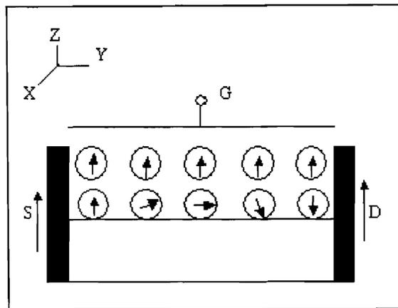
*Figure 5. Schematic of Datta–Das Spin FET.*
