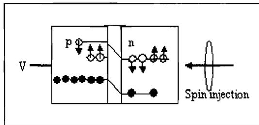
Thus the forward current is modified depending on the sign of the non-equilibrium polarization in the n region. If the polarization is created by circularly polarized light then the open circuit voltage in the diode will depend on the direction of the circular polarization. This is called the spin-voltaic effect. Alternately the short circuit current will show giant magneto-resistance. However practical MBDs are still to be made and tested.
