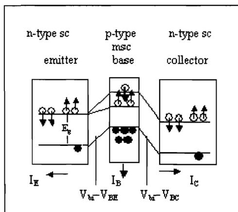
**Figure 4. Schematic for a Magnetic Bipolar Transistor.**
