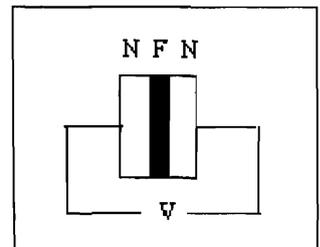
An MBD consists of a diode made of a p-type magnetic semiconductor and a n-type semiconductor. Its I-V characteristic depends on the polarization of the electrons.
