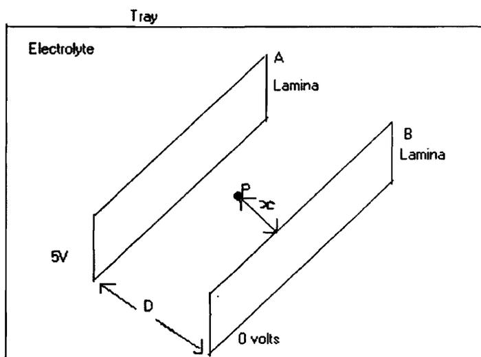
*Figure 1. An electrolytic tank model with two brass laminae A and B separated by a distance D.*
