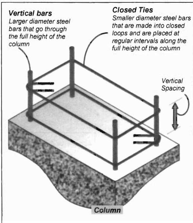
**Figure 1. Steel reinforcement in columns – closed ties at close spacing improve the performance of columns under strong earthquake shaking.**
