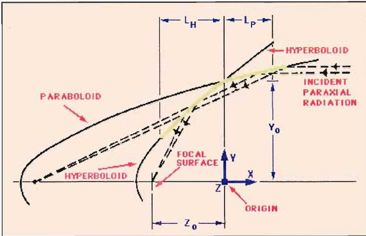
**Figure 2.** A Wolter type I telescope consisting of coaxial and con-focal paraboloid and hyperboloid. This geometry was used in the *Einstein*(NASA), *ROentgenSAT* (Germany, USA, UK), and the *Chandra X-ray Observatories* (CXO) launched by NASA in 1978, 1990 and 1999, respectively.
