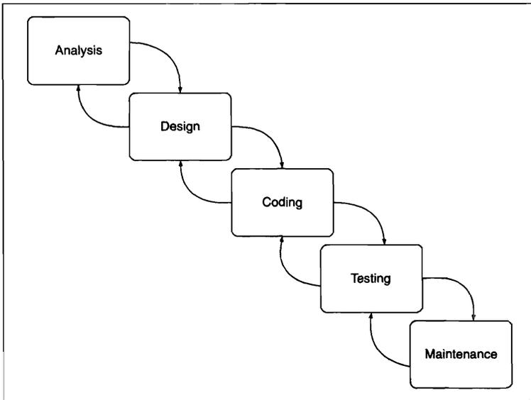
**Figure 1. Waterfall model of software development life cycle.**
