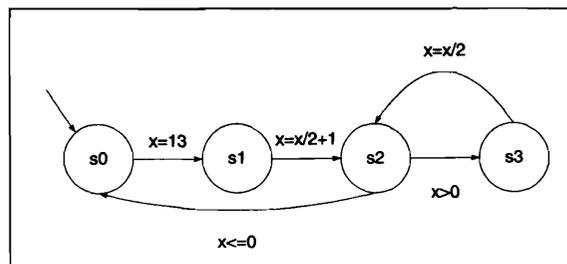
**Figure 3. Model of a simple program.**
