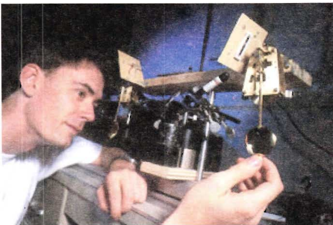
Matthew Bennett adjusts one of the pendulums of the recreated Huygens apparatus.
