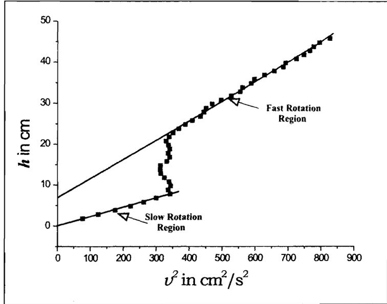
One can measure the length of the tube  $L$ , and the radius of the ball is given as  $r = 1.1 \text{ cm}$ . One obtains  $(L/2 - r)^2 = 338.6 \text{ cm}^2$ . Further simple measurements yield  $2m_0gR^2 = 756 \times 10^3 \text{ g - cm}^3 \text{ s}^{-2}$ . The unknown quantity  $ml^2$  may be written using equation (2) as
