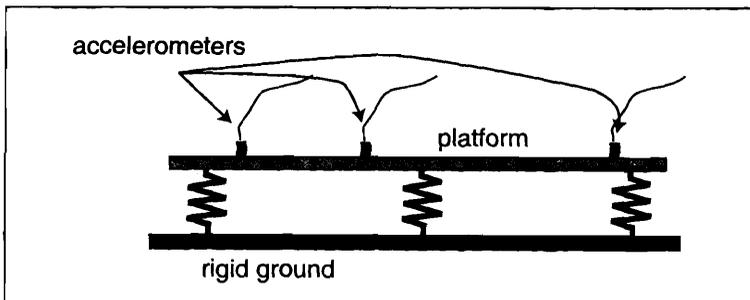
*Figure 1. A vibrating platform.*
