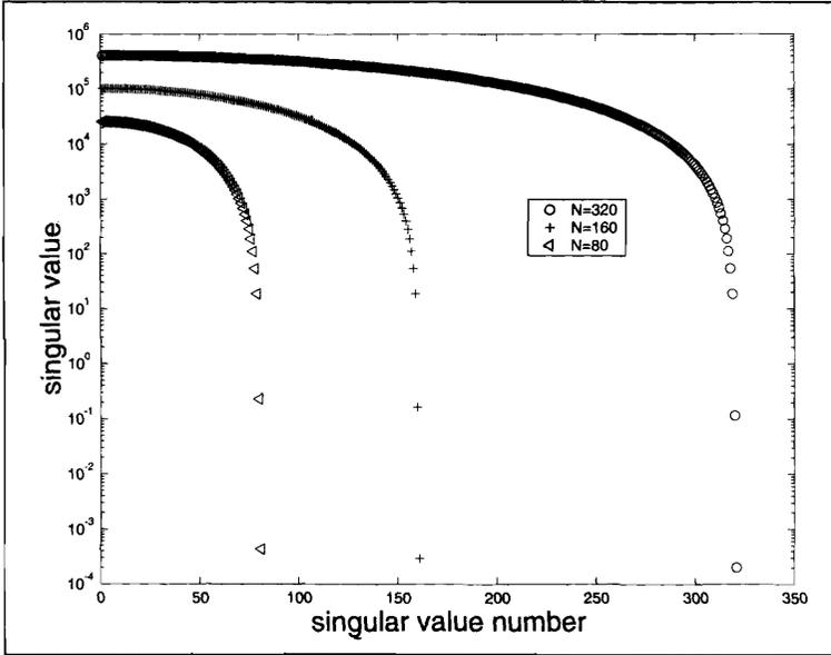
Figure 4. Singular values of *A* from equation (8) for different *N*.
