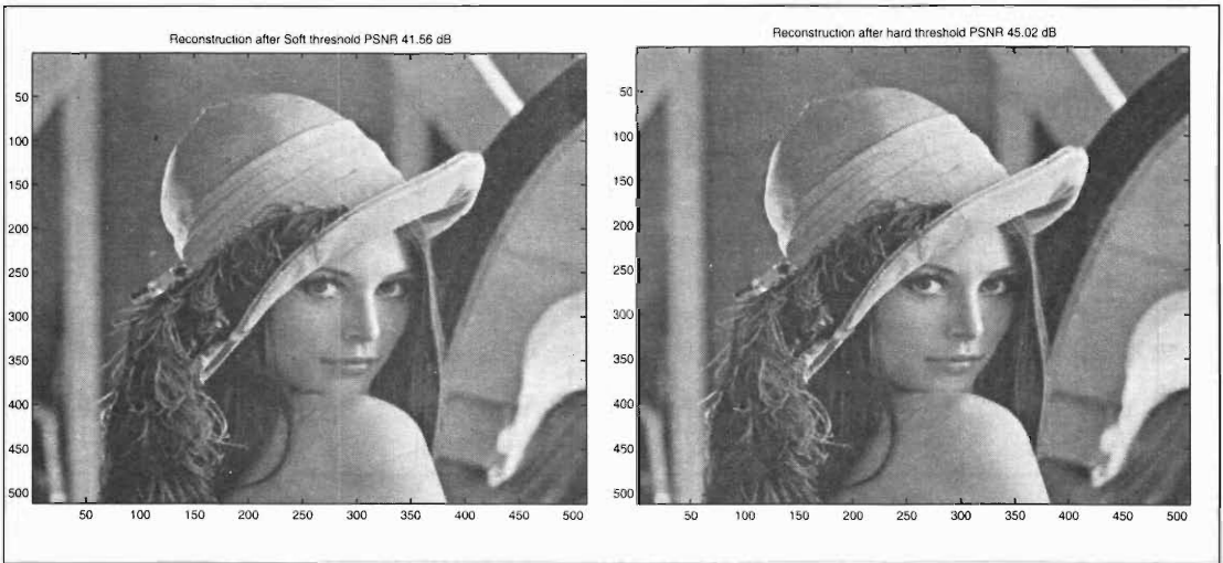
Figure 3. Image reconstruction after soft(left) and hard (right) threshold.
