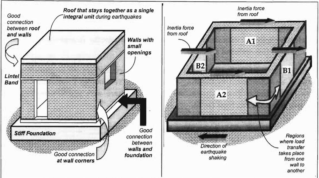
**Figure 1 (left). Essential requirements to ensure box action in a masonry building.**
