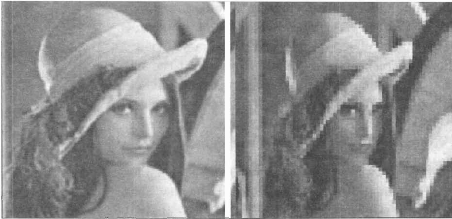
Figure 3. Original image (left) and DCT reconstructed image (right) showing blocking artifacts [9].
