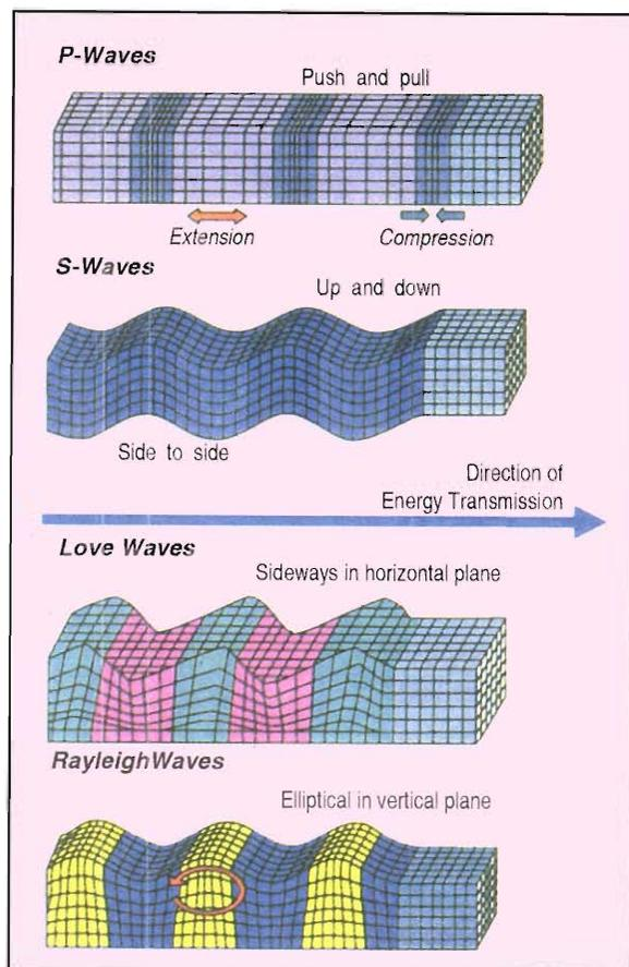
**Figure 2. Motions caused by body and surface waves.**
