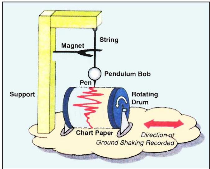
**Figure 3. Schematic of early seismograph.**
