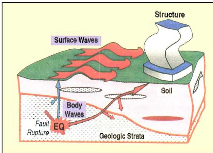
**Figure 1.** Arrival of seismic waves at a site.
