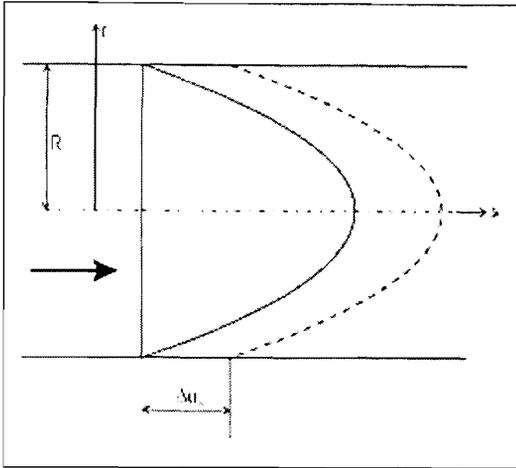
**Figure 3. Parabolic velocity profile in a fully developed pipe flow with and without slip.**
