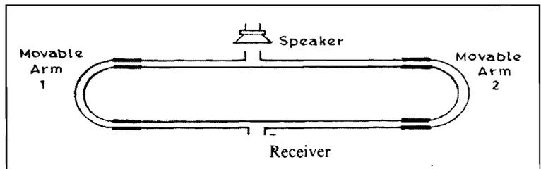
*Figure 1. Quinke's tube setup for measurement of speed of sound in air.*
