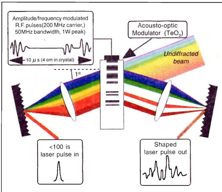
Figure 4. A schematic of the acousto-optic modulated pulse shaping technique.
