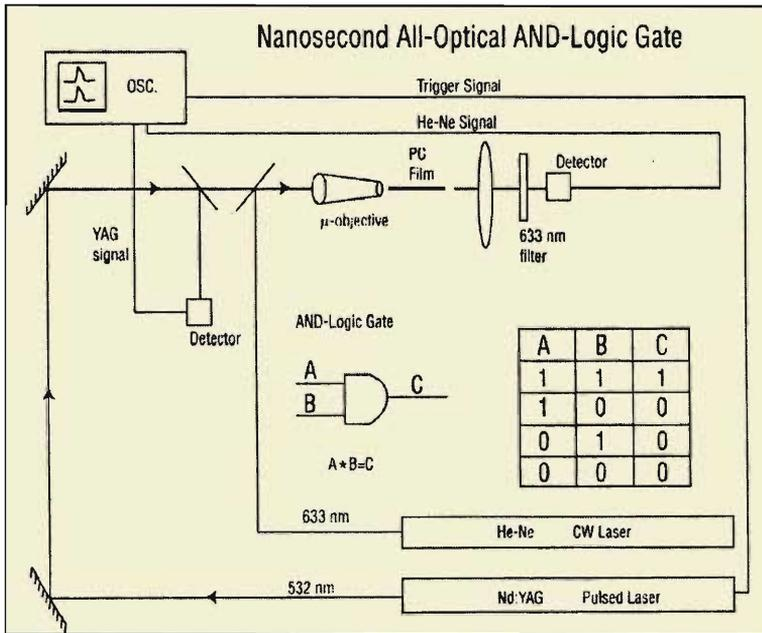
**Figure 1.** A schematic of the nanosecond all-optical AND logic gate setup.
