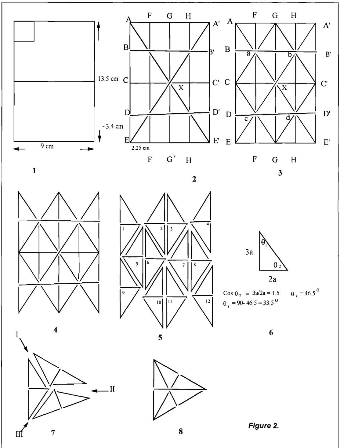
image overlap, by folding along the seam. The joining to the third duplex will, as shown in 7, leave a gap of  $180 - (5 \times 33.5) = 12.5^\circ$ . This is the elegant part of the design, since when the last pair of edges are pasted the center would be lifted up, thus providing the necessary curvature. A planar projection of the module would look like 8 (Figure 2).
