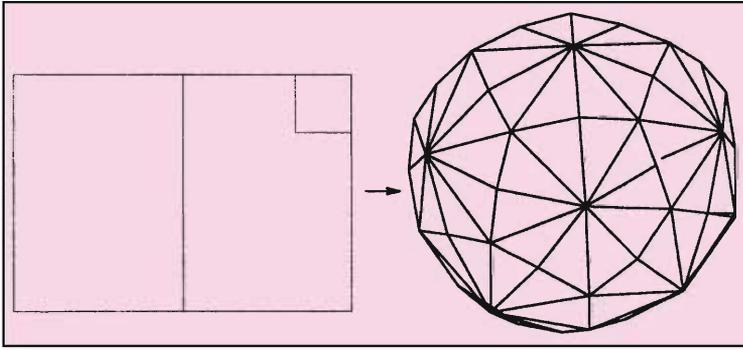
ously in a mirror image fashion with the non-hypotenuse sides in the precise ratio of 3:2. The procedure is illustrated in *Figure 2*.
