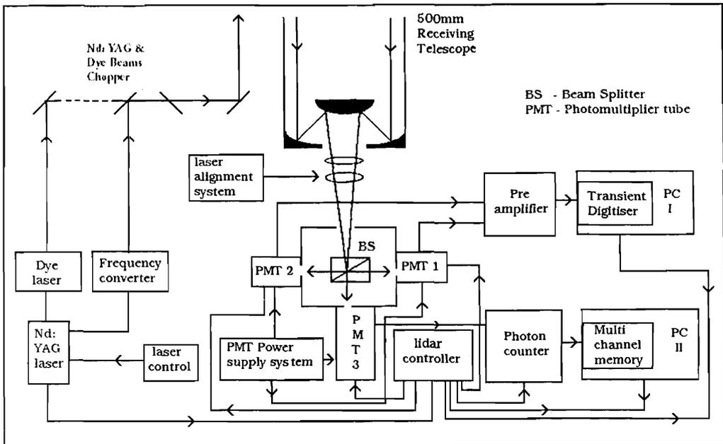
into the atmosphere through a 45° mirror and a 100 mm refracting telescope (only for higher altitude studies). The backscattered radiation is collected by 500 mm Cassegrain receiving telescope. Using a post optics system, the received signal is delivered to the photo multiplier tubes. Interference filters with a bandwidth of 1 nm are used in the post optics to reduce the background noise. The receiver has three channels to cover different wavelength regions and the two data acquisition modes.
