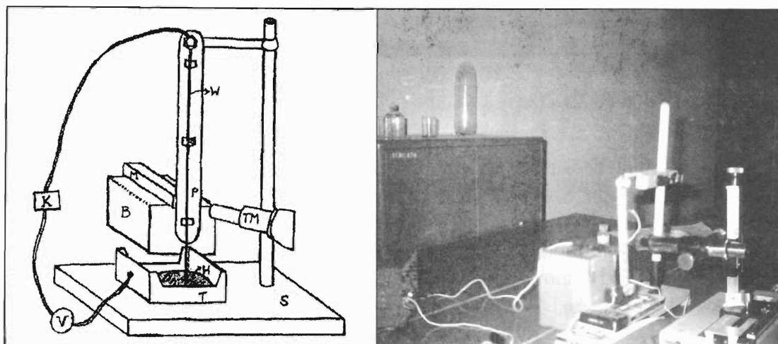
**Figure 1 (left).** Schematic diagram of the set-up. *K*: key, *V*: voltage source, *W*: wire attached to the frame, *M*: magnet, *H*: mercury, *B*: Base, *P*: plastic frame, *T*: trough, *S*: stand, *TM*: travelling microscope.
