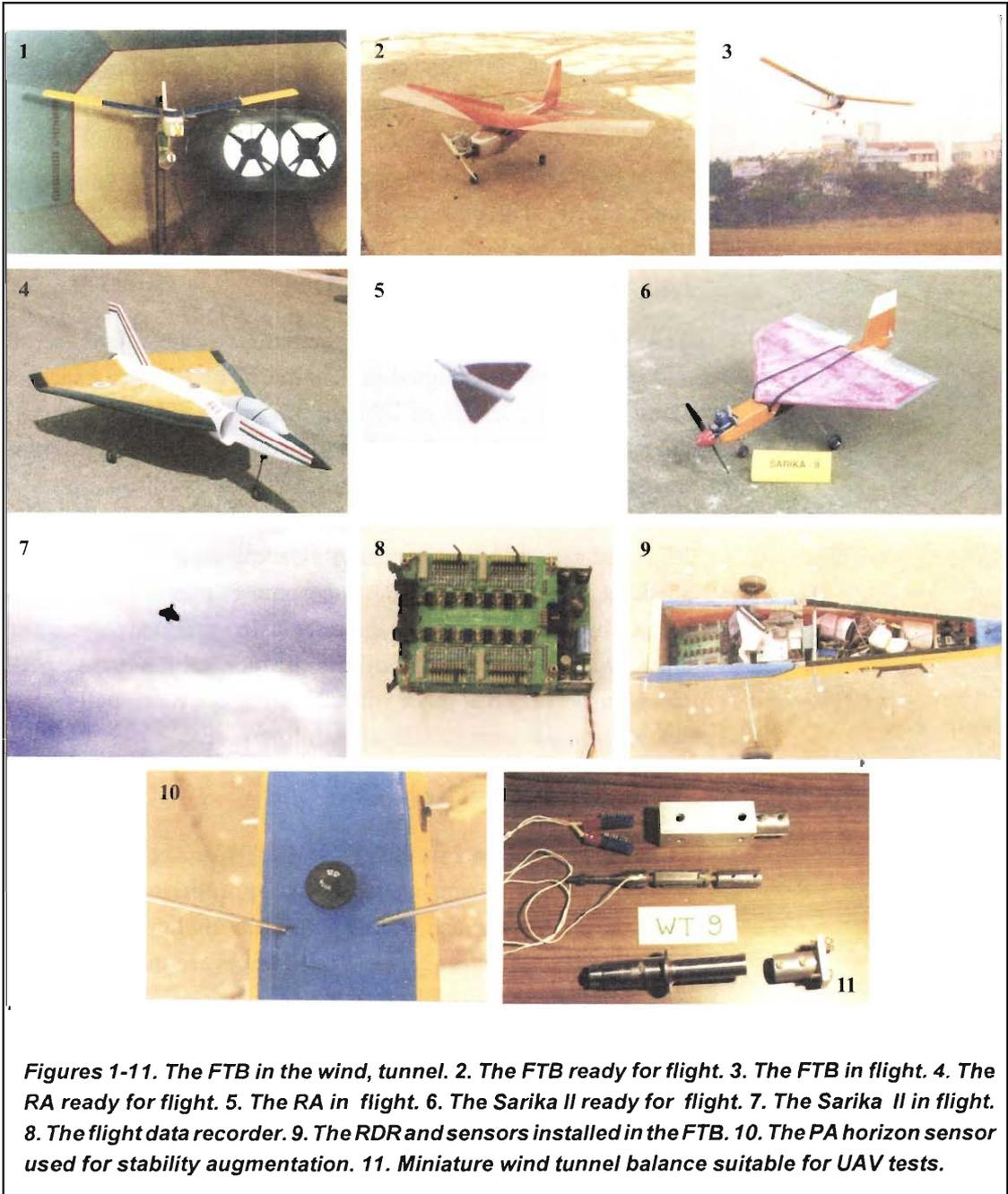
**Figures 1-11. The FTB in the wind, tunnel. 2. The FTB ready for flight. 3. The FTB in flight. 4. The RA ready for flight. 5. The RA in flight. 6. The Sarika II ready for flight. 7. The Sarika II in flight. 8. The flight data recorder. 9. The RDR and sensors installed in the FTB. 10. The PA horizon sensor used for stability augmentation. 11. Miniature wind tunnel balance suitable for UAV tests.**
