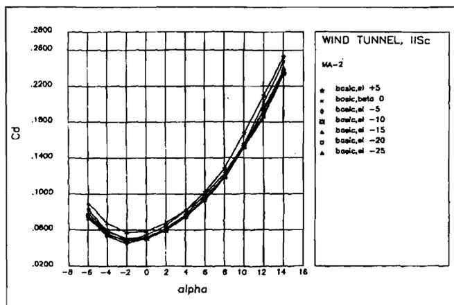
Figure 13. Typical wind tunnel data  $C_D$  vs  $\alpha$ .
