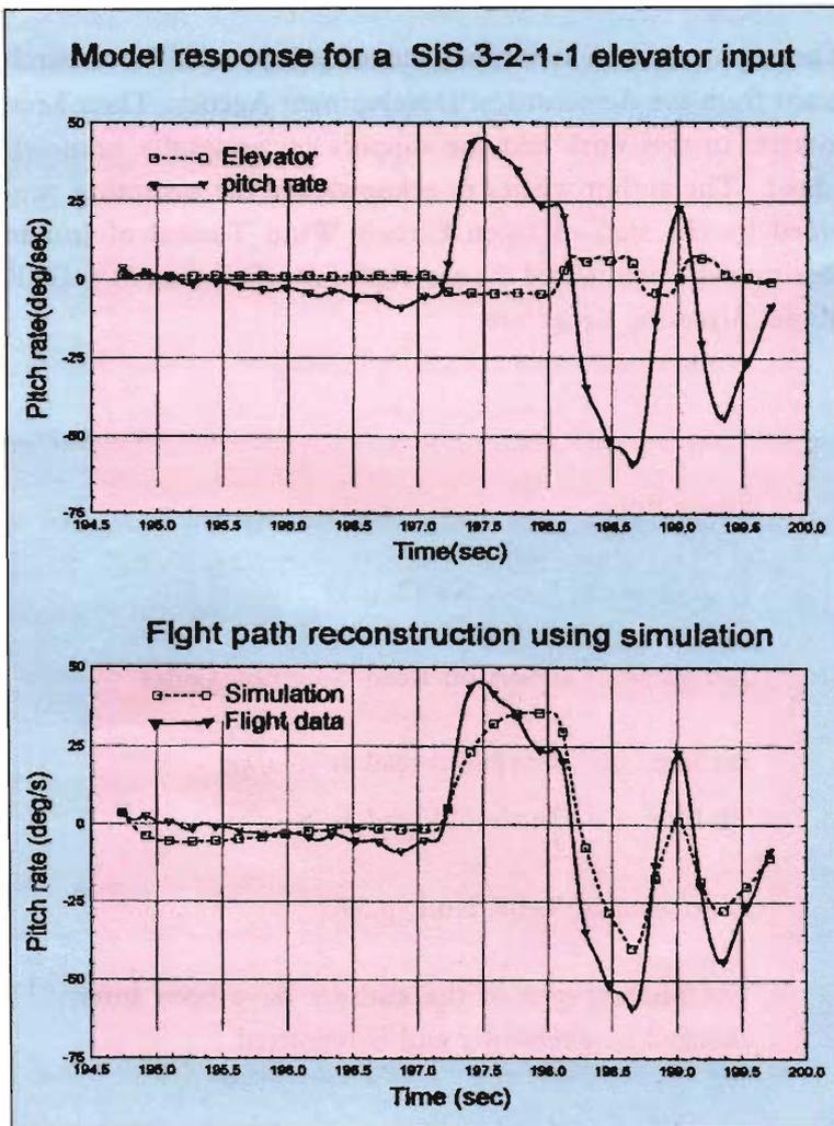
Figure 17. Typical flight results using SIS.
