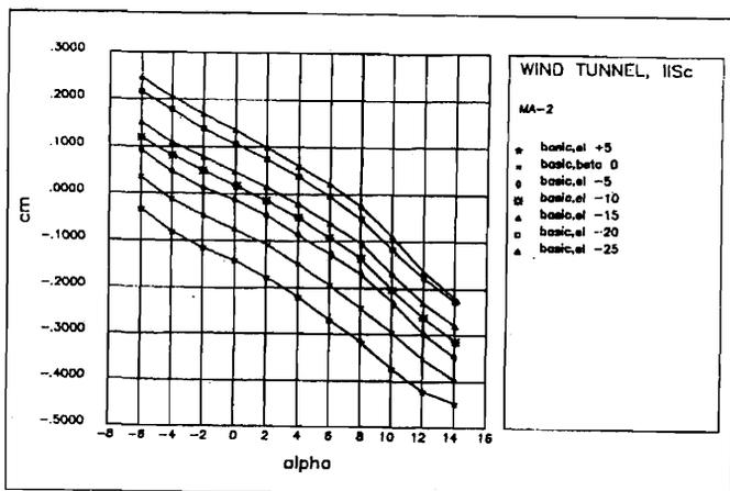
Figure 14. Typical wind tunnel data  $C_m$  vs  $\alpha$ .
