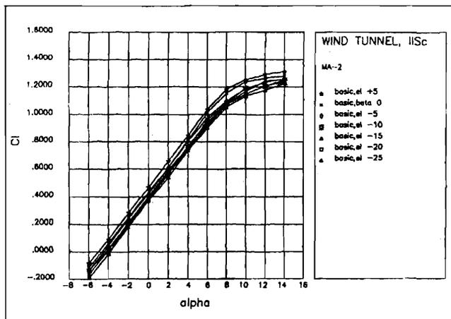
Figure 12. Lift coefficient ( $C_l$ ) variations with angle of attack ( $\alpha$ ).
