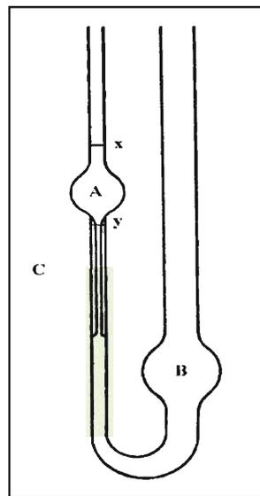
Figure 1. The Ostwald viscometer.
