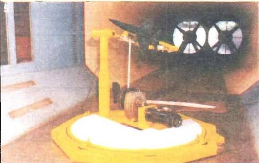
*Figure 1. An aircraft model mounted on sting type balance.*
