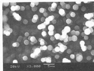
Figure 14. SEM image of amorphous carbon film.
