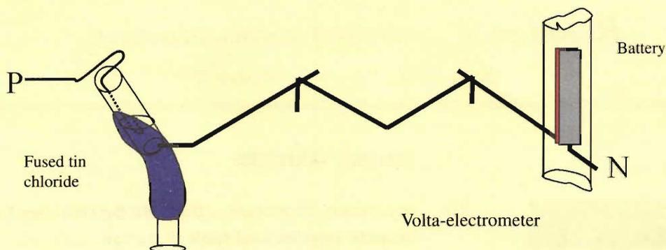
*Apparatus used for the determination of chemical equivalent of tin. Fused tin chloride is electrolyzed using an electrolysis cell with two electrodes. The difference in weight of the cathode before and after the deposition of the metal is used to determine the chemical equivalent. The electricity passed through the cell is determined using a volta-electrometer.*
