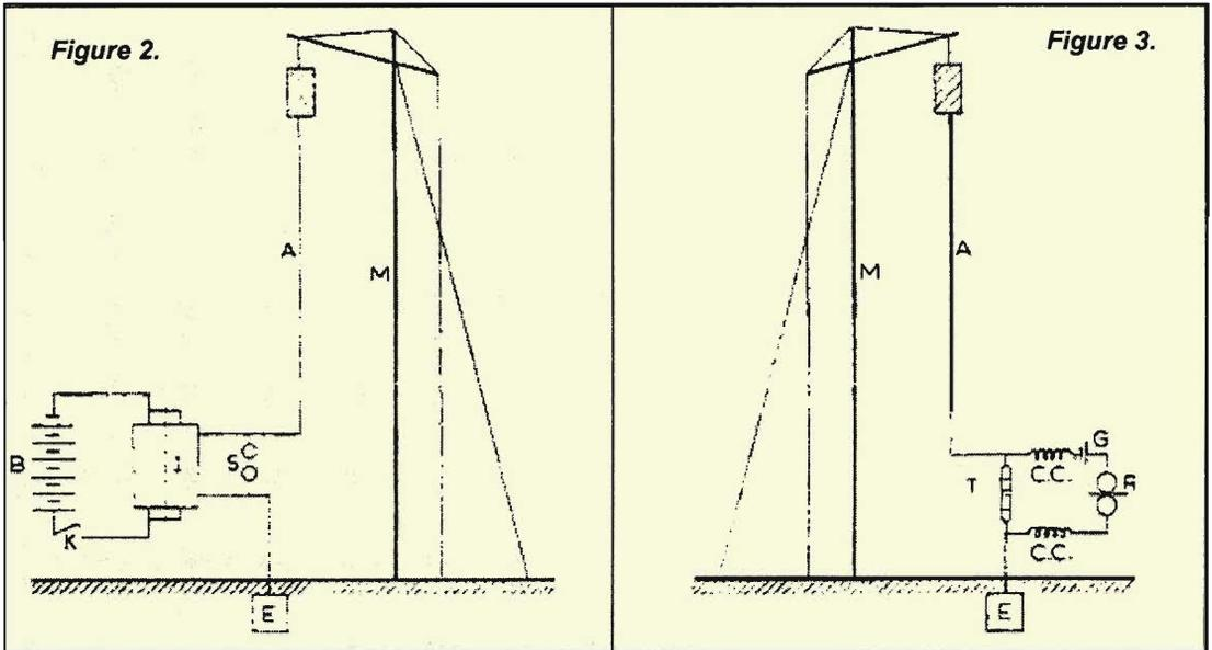
the distance over which it was possible to telegraph. Thus I found that when using cubes of tin of about 30 cm side as elevated conductors or capacities, placed at the top of poles 2 meters high, I could receive signals at 30 meters distance, and when placed on poles 4 meters high, at 100 meters, and at 8 meters high at 400 meters. With larger cubes 100 cm side, fixed at a height of 8 meters, signals could be transmitted 2,400 meters all round.
