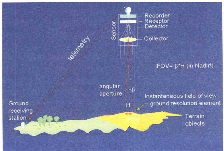
**Figure 1.** Shows schematically the principle of remote sensing.
