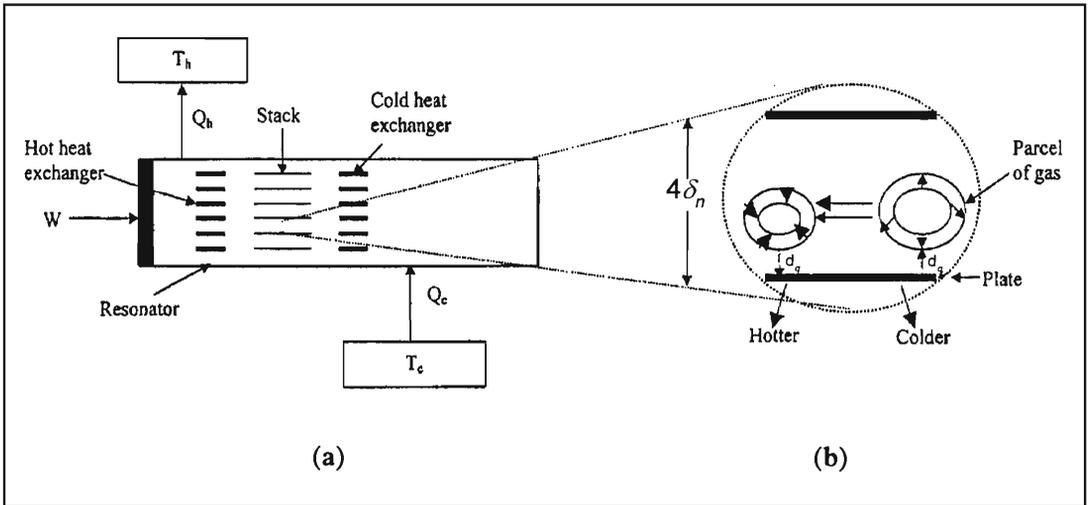
**Figure 1. Schematic diagram of a thermoacoustic refrigerator module.**
