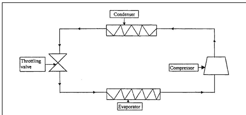
**Figure 1. Schematic diagram showing the mechanical refrigeration system.**
