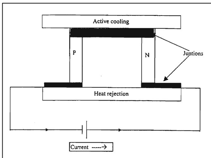
in the device because electrons carry heat, and 'hot' electrons can be forced away from the cold end of the device by the battery.
