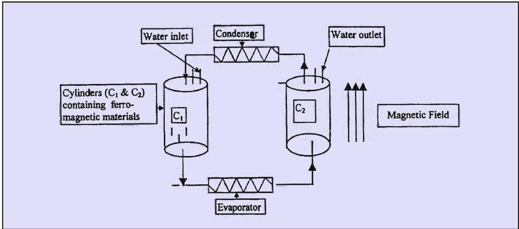
**Figure 2. Schematic diagram showing the magnetic refrigerator.**
